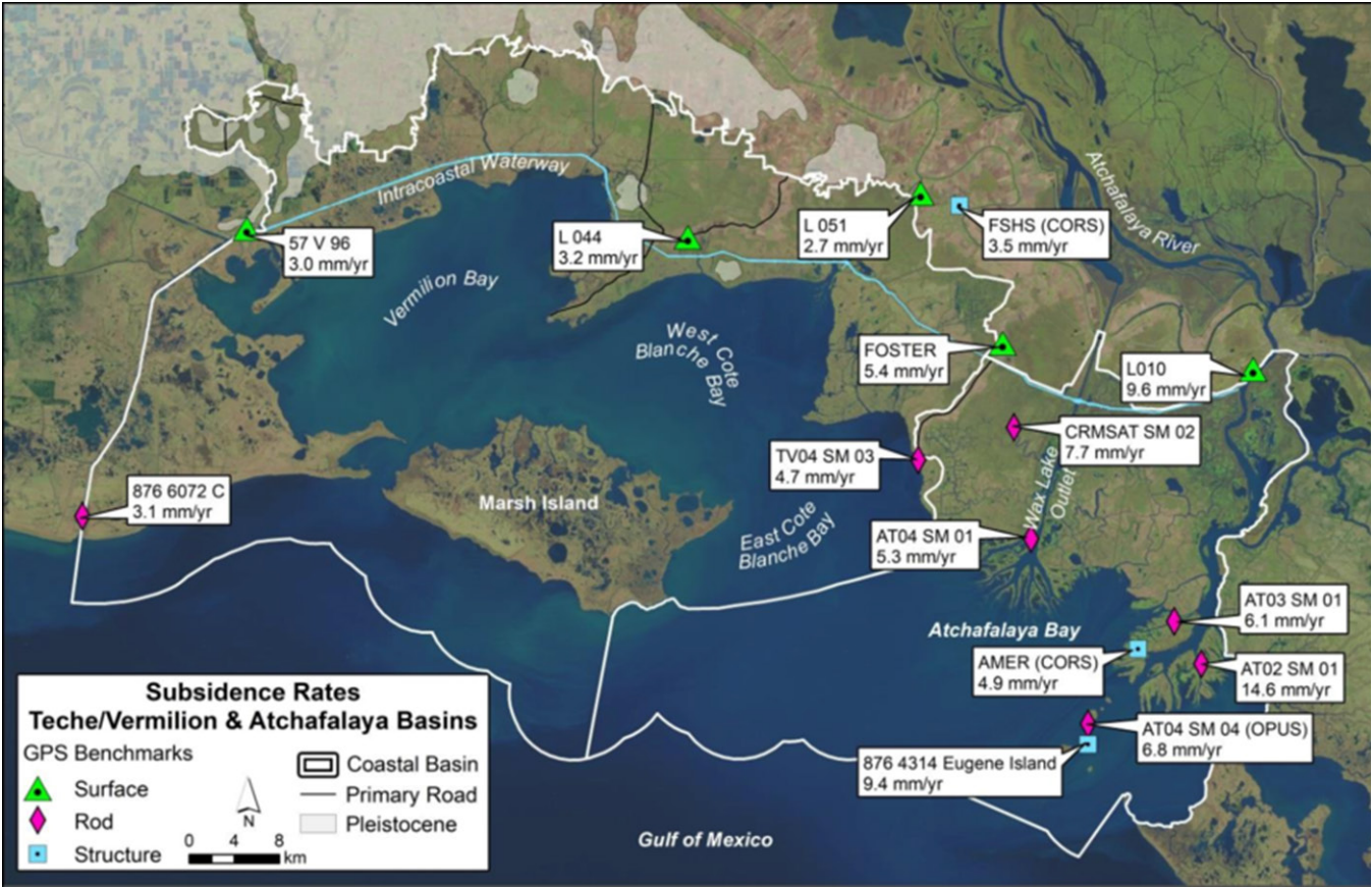
Figure 18. Subsidence rates (mm/yr) for primary and secondary benchmarks for Teche/Vermilion and Atchafalaya Basins demonstrate high subsidence velocities near the Atchafalaya River and Wax Lake Outlet. Background image: Landsat 8 OLI/TIRS, acquired Nov. 6, 2021.
